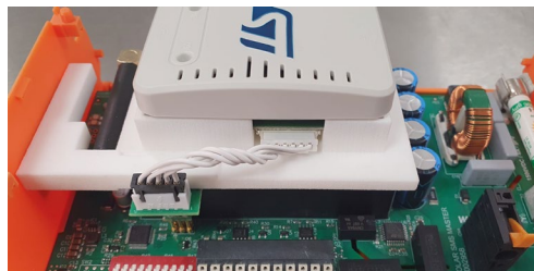
Figure 9: Correct positioning of the SOLAR SMS MASTER & MASTER LORAWAN STLINK FIELD UPGRADING KIT (jig) and its pins over the DC/DC converter
