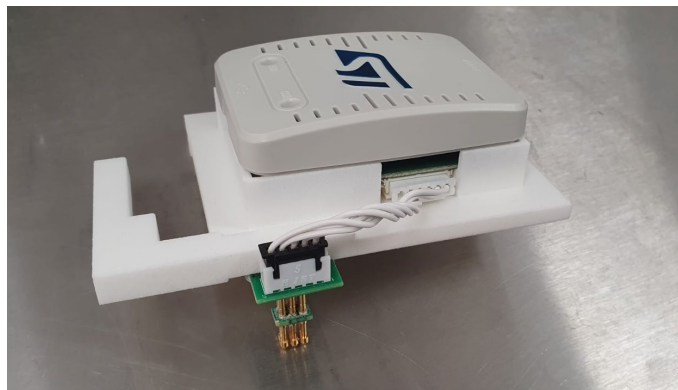
Figure 4: SOLAR SMS MASTER & MASTER LORAWAN STLINK programming jig
